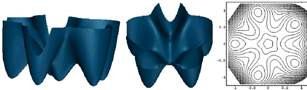
Figure 3. Various views (left and centre) and a contour line map (right) of the free energy landscape of the 'jello-mould' type model by Morin et al (1995). The central minimum represents the liquid, while the other minima correspond to different crystallographic orientations. (The phase field is the radial distance from the centre, and the angle is the orientational variable.)
